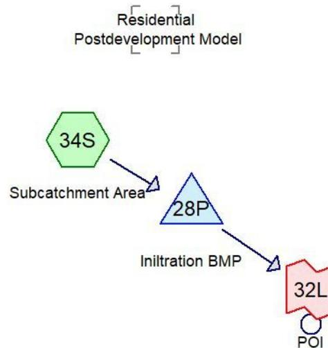
*Figure 7: Model of stormwater flow at design site*
