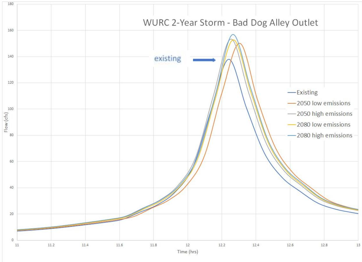
Figure 7. Modeled runoff for the 2-year storm for example area using existing and projected storm events.
