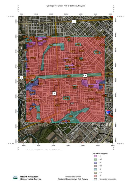
Figure 8: Natural Resource Conservation Service Web Soil Survey Map for hydraulic soil group.
