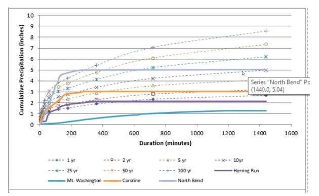
Figure 2: Precipitation - duration at several monitoring locations for the August 22, 2019 event compared with 24-hour Design Storms (BCDPW).
