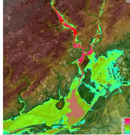
Figure 1. Flood modeling including both rainfall and storm tide in Philadelphia. Example of Hurricane Sandy storm surge combined with Hurricane Irene type streamflow.
